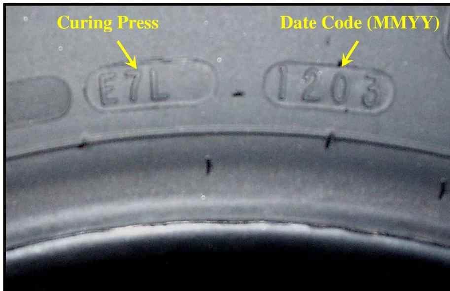
On the sidewall near the bead area, there is a six digit number followed by a hyphen and a seven character code. The first six digit number refers to the mold piece number and the seven character code is the mold code. The mold code refers to the size and shape of the mold used and the piece number refers to the specific mold the tire was cured in. Therefore, all tires with the same D number will have the same mold code, but can have different piece numbers.
